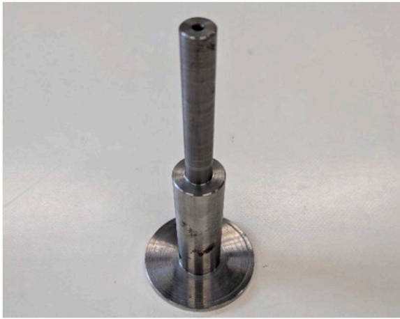
. 7. Steel pipe pile with 64 mm expanded base wing.
