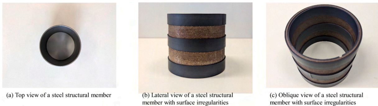
Fig. 5. Steel structural members with surface irregularities.
